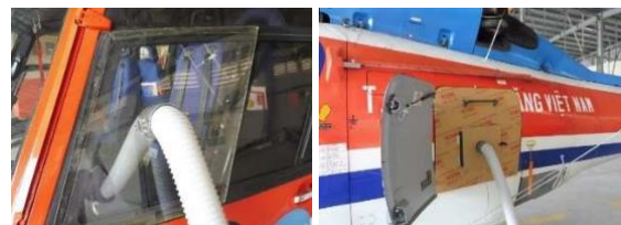
Fig. 5. Connecting dry air pipeline to the cabin and the cargo compartment of the helicopter through «fake» windows
