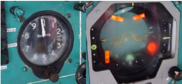
Fig. 3. Vapor condensation inside the helicopter's indicators
